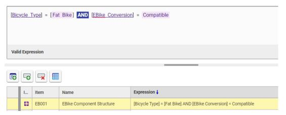
This Usage Condition will configure the structure to show EBike components only when Bicycle Type is 'Fat Bike' and EBike Conversion is 'Compatible'.
